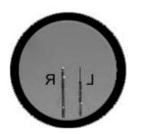
Choose a distant object that is at least 500 meters (or yards) away and point the main telescope at the object. Adjust the telescope so that the object is in the center of the view in your eyepiece.
